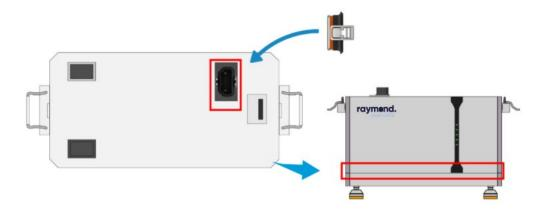
Turn on the Breaker: Breaker is on the top of the battery covered by a panel, open the panel. Turn on the Breaker and install the panel again.
